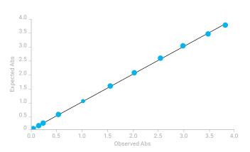
Superior accuracy and photometric linear range The photometric range of the Cary 60 extends above 3.5 absorbance units. As shown above, a correlation coefficient of 0.999 was achieved when measuring certified standards (Starna, S/N 14727, set type RM-9ND). The absorbance was measured at 525 nm using
