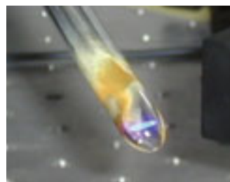
Fig. 11: Indium cell with blue fluorescence.
